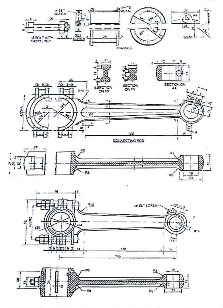
on: Assemble the parts and draw the following views of it: (a) front view upper half in section and view full in section.
