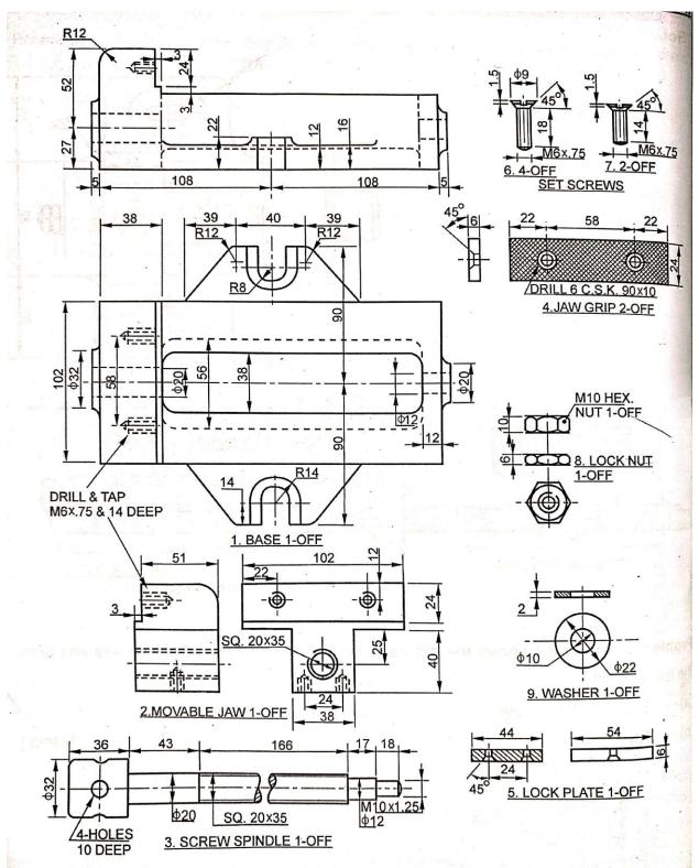
**Figure** shows details of Machine Vice. Assemble the parts and draw the following views:-(a) Sectional front view (b) Top view
