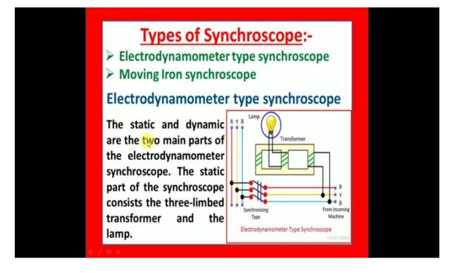
The winding of the outer limb of the transformer induces two flux. And the flux of the central limb is the resultant of the outer two limb flux. The resultant flux induces the EMF in the central winding of the transformer.
